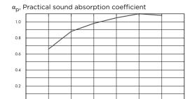
Eurocoustic Tonga® Therm A, 200 mm o.d.s.o.d.s = overall depth of system
